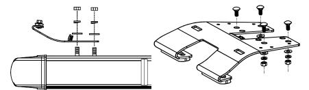
8. Using two people, carefully place the lightbar on the vehicle roof and locate it in a position which is level front to back, and is centered side to side. The area above the B-pillars is often used, since it is usually the strongest part of the roof. Slide the bracket outwards so that the rubber feet are as close to the edge of the roof as possible. Tighten the hex nuts on the carriage bolts to secure the mounting brackets in position.
