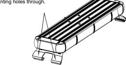
2. Carefully remove the bar and drill the appropriate holes in mounting surface, taking care not to drill through the headliner (if applicable).
