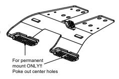
4. Turn the lightbar over to access the channels along the bottom of the lower extrusion, taking care not to scratch the lenses and or your vehicle. Install the eight carriage bolts into the channels running underneath the lightbar by inserting the heads in the center hole.
