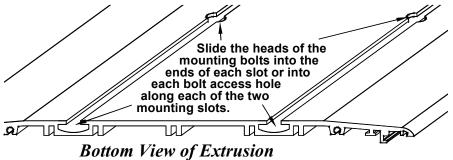
5. Slide two bolts in each channel towards both ends. You will use four bolts on each end (two in each channel) to secure each mounting bracket.
